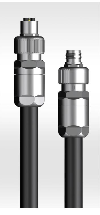
The PROVERTHA M12 Power connectors with L-Codierung 4+ PE are standardized in the IEC 61076-4-111. The PROVERTHA M12 Power connectors characterised by a full metal housing and the vibration-proof crimp techology for the power contacts. The connectors are designed for a wide cable clamping range für cables with wire sizes up to 2,5 qmm and outer diameters up to 14 mm. The connectors are the right solution for applications with
